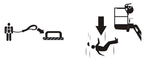
• Keep both feet firmly positioned on the platform floor at all times. Never use ladders, boxes, steps, planks, or similar items on platform to provide additional reach.
