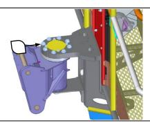
Check if there is some bolts is slacken or missing and the sensor undamaged. If there is abnormal condition, ask for help from dingli or your agency.
