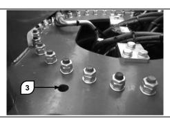
To check the fixing screws of the slewing ring gear on the chassis, align hole **3** with the screw underneath by rotating the turret.
