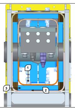
3) Slacken all the bolt 1 of the upper and lower sliding blocks of the first extension stage. If the space between the sliding surface of the block 3 and the sliding surface of the first boom exceeds 0.5mm, some pads 2 need to be added. And then tighten bolts 1.
