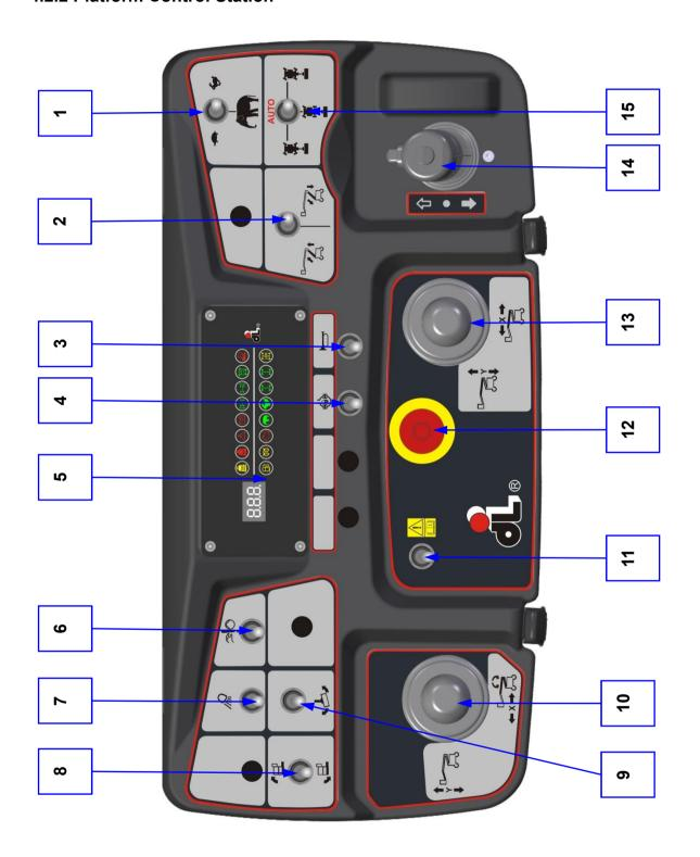
Figure 4-2 Platform Console Panel
