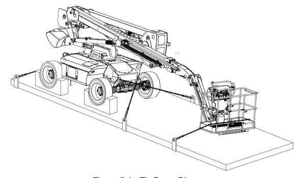
Figure 5-4 Tie Down Diagram
