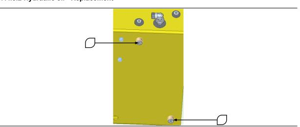
1) Go under the vehicle to access the tanks drainage caps.
