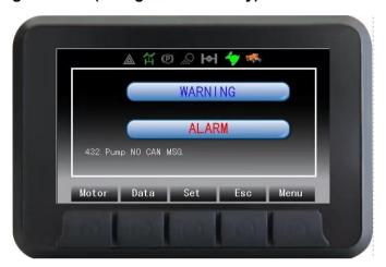
Figure 4-9 Alarm/Warning Interface
