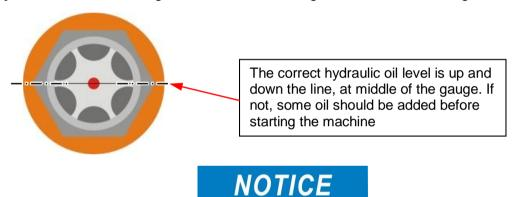
ON NEW MACHINES, THOSE RECENTLY OVERHAULED, OR AFTER CHANGING HYDRAULIC OIL, OPERATE ALL SYSTEMS A MINIMUM OF TWO COMPLETE CYCLES AND RECHECK OIL LEVEL IN RESERVOIR. SOME HYDRAULIC OIL MAY BE NEEDED, THAT SHOULD BE APPLIED TO THE ENVIRONMENT OF THE LOCATION AND FILTERED, WHILE THE FILTRATION ACCURACY IS 20um.
