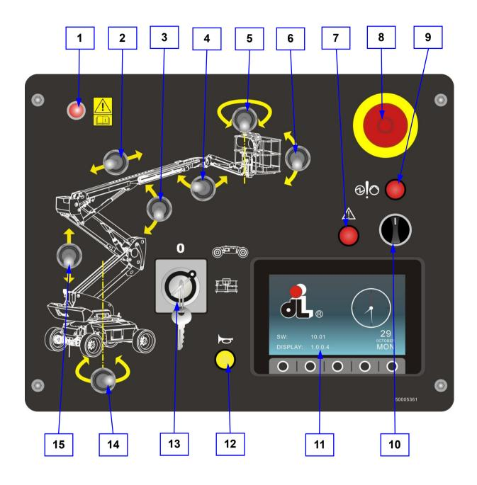
Figure 4-1 Ground Console Panel
