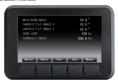
**Figure 4-6 Vehicle Condition Interface**
