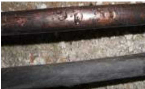
Damaged hydraulic hose pipe
