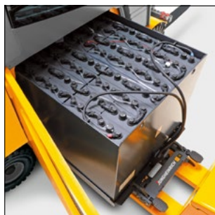
Lateral battery exchange
