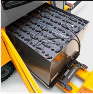
Lateral battery exchange
