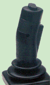
Fig. 6 Joy-stick at the portable control box
