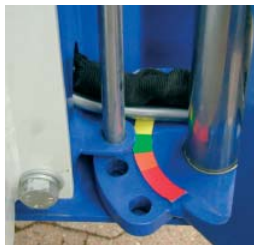
Fig. 17 Outrigger in standard position.
