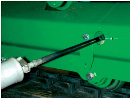
Fig. 67 Grease gun on grease nipple for the tension roller
