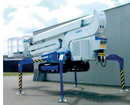
Fig. 58 Platform lifted at the outriggers
