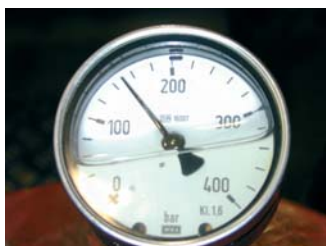
Fig. 68a Pressure gauge on Grease gun
