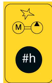
PUSHBUTTON STARTS PUMP FOR OUTRIGGERS
