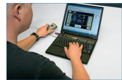
Bronto TeleControl system enables information transfer between the diagnostic system of the aerial and Bronto Skylift Customer Service. Fault analysis and telemaintenance can be performed on-line.
