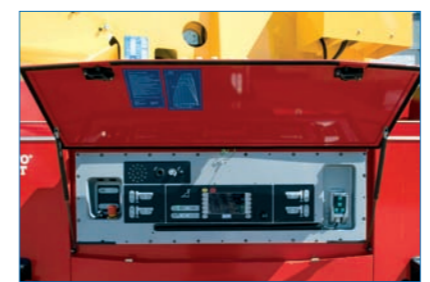
Automatic one button variable jacking.
